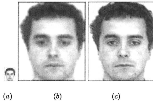
Fig. 7.15. (a) A low resolution observation of different image size 41 \times 48 pixels, (b) bicubic interpolated image with r = 8 and, (c) PCA-based reconstruction.
