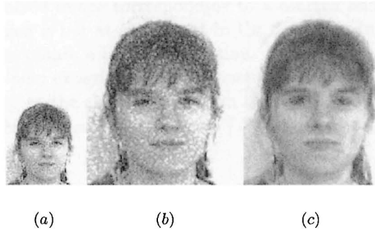
Fig. 7.6. Restoration of an input image not present in the database. (a) Noisy observation, (b) bicubic interpolated image, and (c) result of PCA-based restoration for r = 2 .
